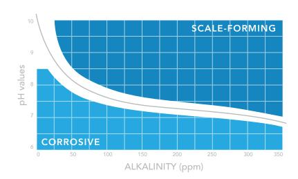
Acid is used to lower pH. An example is hydrochloric acid. This will effectively lower the pH and total alkalinity. If using hydrochloric acid to lower pH, it is vital that it be diluted (one part of acid to ten parts of water) prior to adding to the water. Note that the filter should be running when you add the diluted hydrochloric acid and for at least one hour afterwards to ensure adequate mixing. No other types of acid should ever be used for pH or total alkalinity adjustment.
